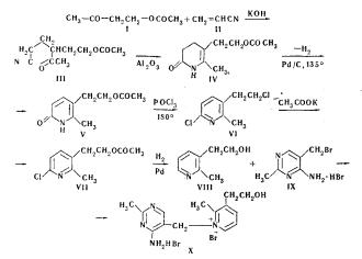
To synthesize 2-methyl-3-( $\beta$ -hydroxyethyl)pyridine (VIII), the pyridine component of pyrithiamine, a condensation was conducted between acrylonitrile and 3-butanonyl acetate (I) with subsequent ring formation of 3-aceto-5-cyano-pentyl acetate (III) into 2-methyl-3-( $\beta$ -acetoxyethyl)-4, 5-dihydropyrid-6-one (IV) according to a previously described method [2].
